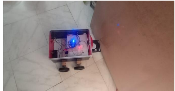
Fig. 7 Ultrasonic sensor detects the obstacle and pulls the bumper to avoid the damage
